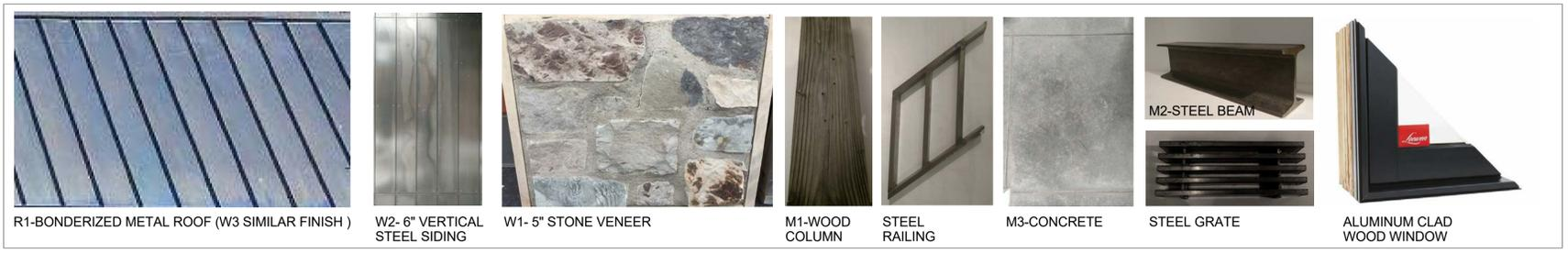
R1-BONDERIZED METAL ROOF (W3 SIMILAR FINISH) W2-6" VERTICAL STEEL SIDING W1-5" STONE VENEER M1-WOOD COLUMN STEEL RAILING M3-CONCRETE STEEL GRATE ALUMINUM CLAD WOOD WINDOW
