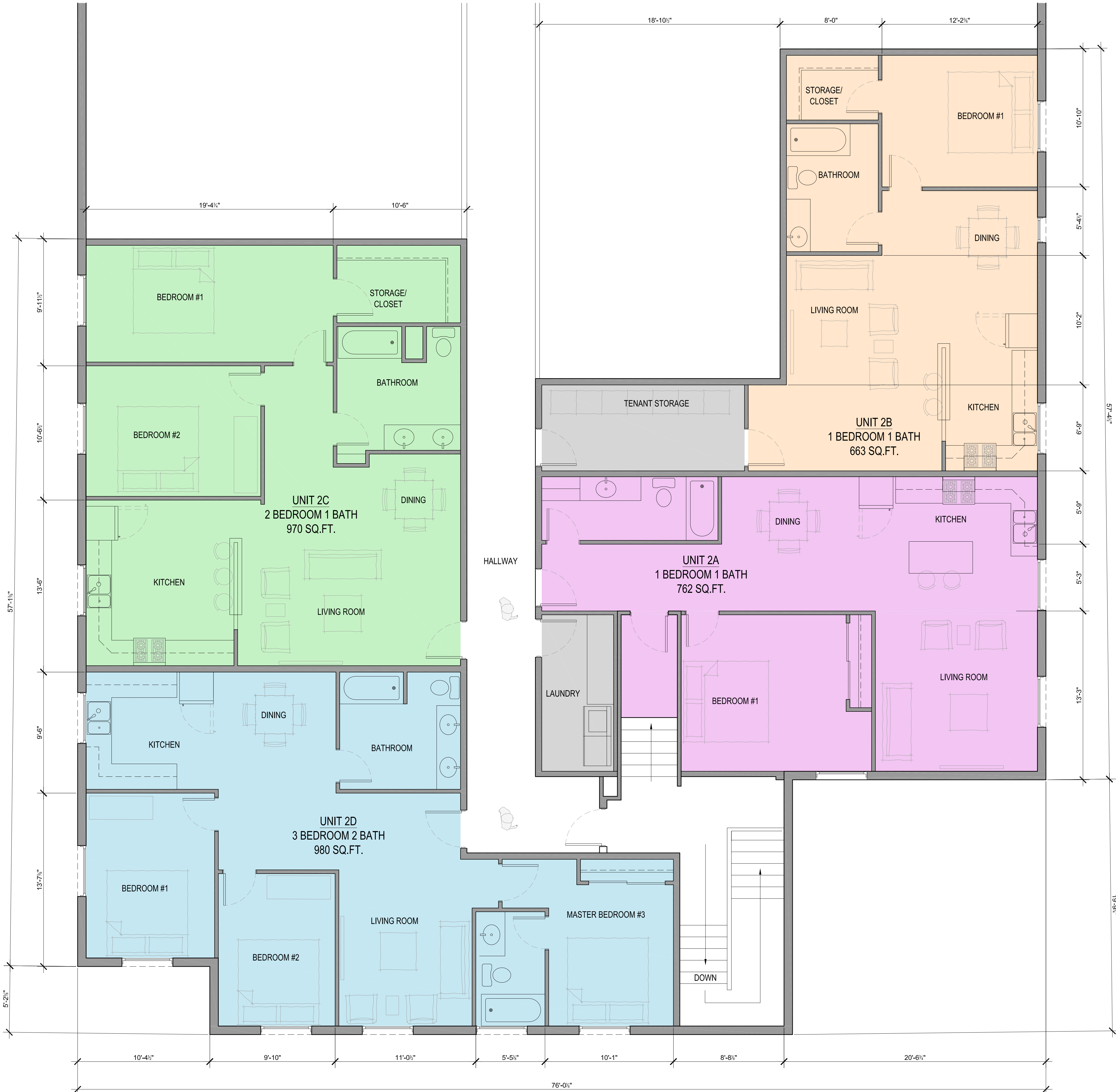
PROPOSED SCHEMATIC FLOOR PLAN - V1 (1 bedroom unit 2A)
