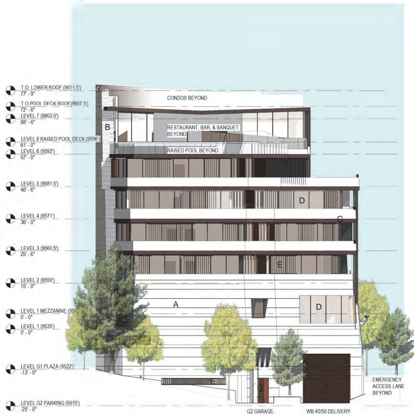
3 WEST MATERIAL ELEVATION 1/16" = 1'-0"
