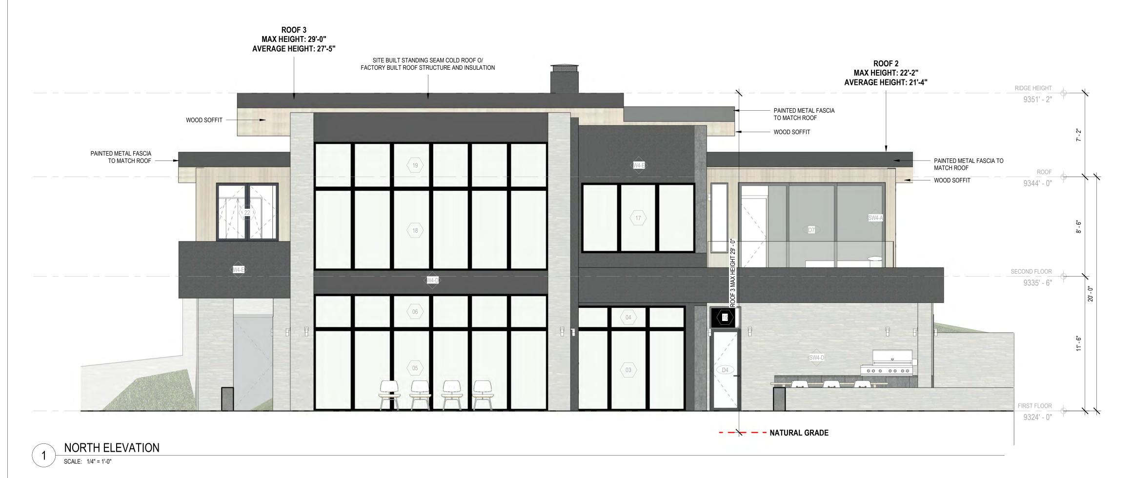
ROOF 3 MAX HEIGHT: 29'-0" AVERAGE HEIGHT: 27'-5" PAINTED METAL FASCIA TO MATCH ROOF ROOF 2 MAX HEIGHT: 22'-2" AVERAGE HEIGHT: 21'-4" 9351' - 2" SITE-BUILT ROOF SITE BUILT STANDING SEAM COLD ROOF O/ FACTORY BUILT ROOF STRUCTURE AND INSULATION ROOF 9344' - 0" PAINTED METAL FASCIA TO MATCH ROOF ROOF 1 MAX HEIGHT: 14'-2" AVERAGE HEIGHT: 12'-4" SITE-BUILT ROOF <SW4-A> SECOND FLOOR 9335' - 6" SW4-E FIRST FLOOR 9324' - 0" \_ \_ \_ \_
