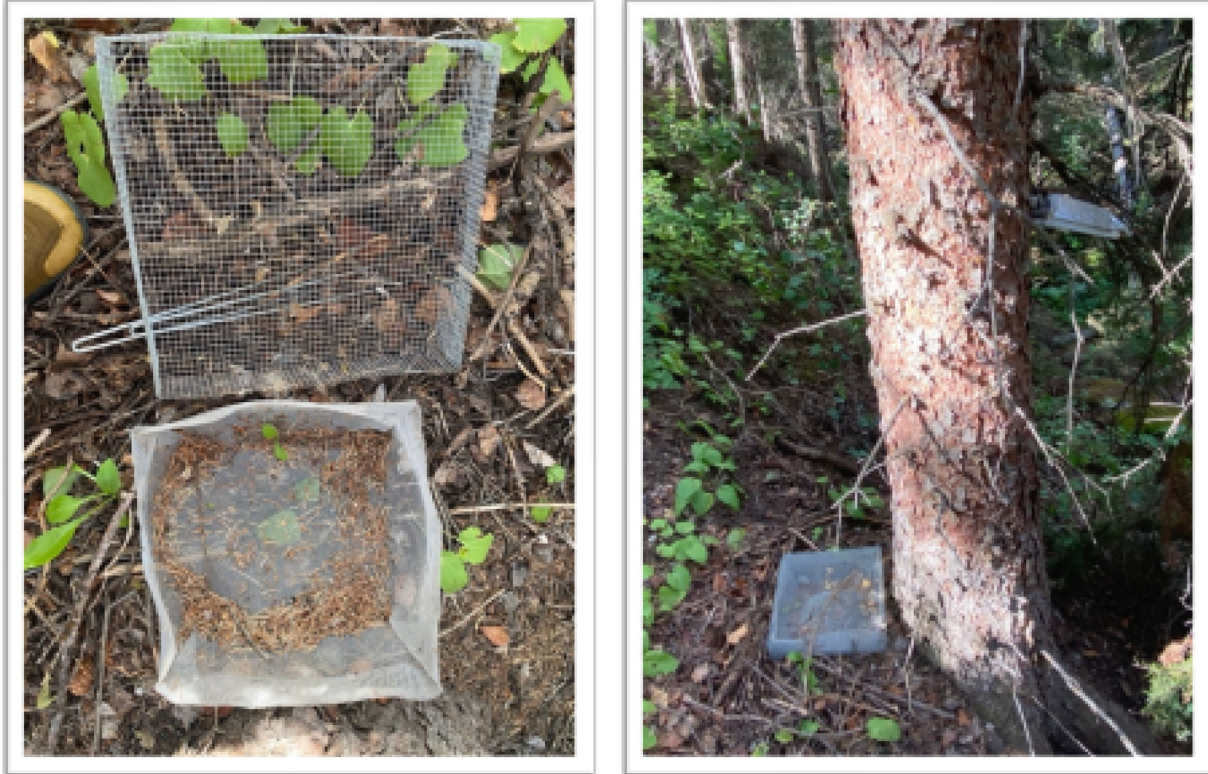
Figure 2. Seed trap from forest monitoring plot #9 from August 2023. Leg: the bottom (fine mesh) and top (coarse mesh, and landscaping pins). Litter inside fine mesh was the collection of material between summer 2022 and summer 2023. Right: The seed trap shown in the leg photo deployed in plot #9 at the base of a spruce tree. Note: the silver box attached to the right side of the tree is a solar radiation shield with a temperature sensor, which is constantly recording temperature at the site and can be valuable to relate weather changes to forest dynamics (e.g., spruce seed production, seedling establishment, insect activity).
