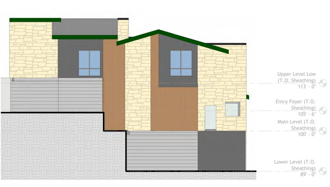
2 SOUTH ELEVATION - MATERIAL CALCULATIONS 1/8" = 1'-0"
