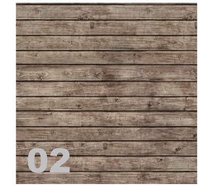
02 WOOD SIDING: 6" horizontal SPF (spruce, pine, fir mix) wood siding
