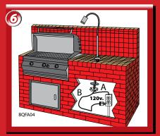
6: A: Hard wire directly into internal J-Box supplied within built in BBQ B: If receptacle is present, attach a grounded mechanical plug and simply plug in **Commercial Mount Barbecues**
