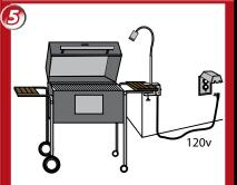
5: Plug 9' grounded powercord into weatherproof receptacle via power cord (supplied by Focus)
