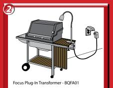
2: Plug-in 12v transformer to 120v receptacle with 10' 18/2 SPT-1W black lead wire
