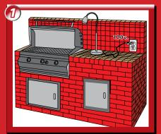
1: Plug 9' grounded powercord into weatherproof receptacle via power cord (supplied by Focus)
