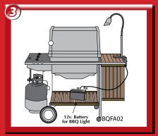
3: Quick connect to 12v rechargeable/portable battery with 10' 18/2 SPT-1W black lead wire
