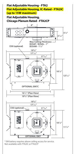
available with each housing increase maximum accepted ceiling thickness. -15accepts 1.5" max ceiling thickness adds 0.5" to overall housing height reduces light output by 20%
