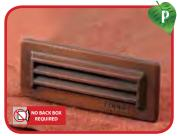
12v Driver Supplied SLO8LEDPBAR: NO BACK BOX REQUIRED Cast aluminum or brass 12v 8w integrated flat panel LED 50,000 hours average rating 3000K warm white or 5200K cool white External 12v AC driver required (supplied)
