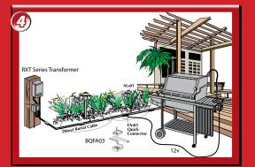
4: Direct connection to 12v. landscape lighting system with supplied FA-05 Quick Connector with 20' 18/2 SPT-1W black lead wire
