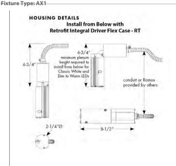
FIELD REPLACEABLE LED LIGHT ENGINE is serviceable through the aperture with a Phillips screwdriver.
